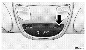
Use this button to select a readout of the outside temperature and one of eight compass headings that indicate the direction in which the vehicle is facing.
